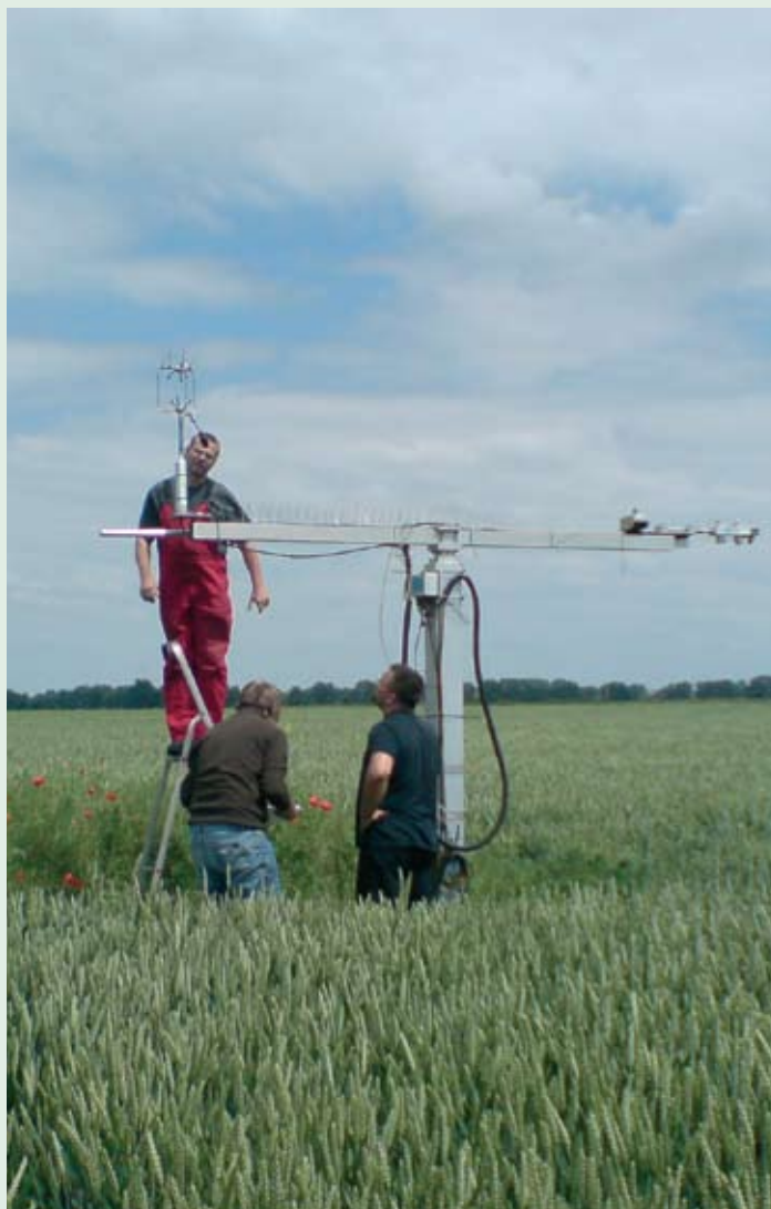
Fig 24: Maintaining eddy flux instruments over a crop field. (Photo: W. Ziegler)
