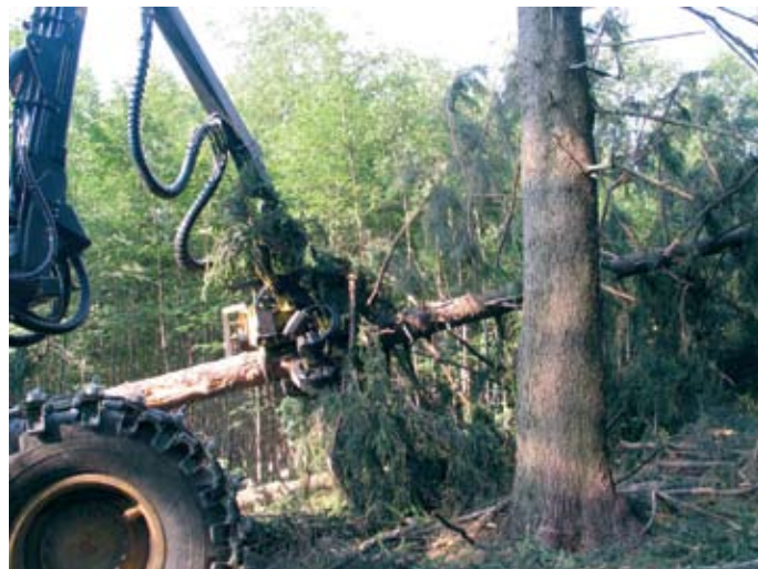
Fig 11a: The wood is harvested by heavy machinery. The harvester fells the tree and cuts it into pieces. (Photo: E.-D. Schulze)
