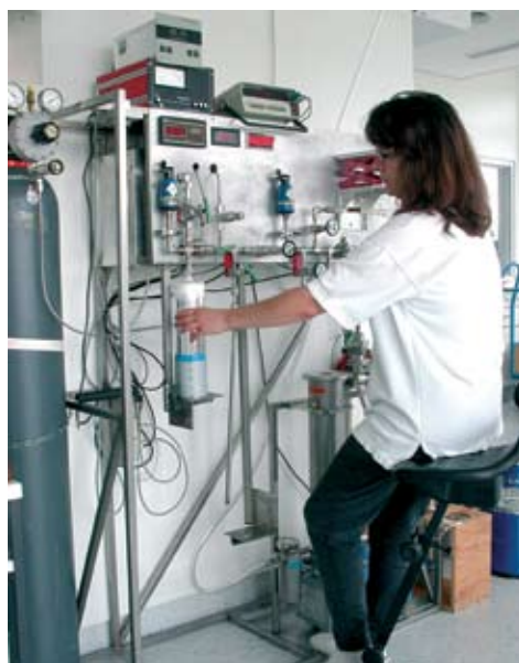
Fig. 57: Technician preparing 14 CO 2 sample for counting in the Heidelberg Radiocarbon Laboratory. (Photo: B. Kromer)
