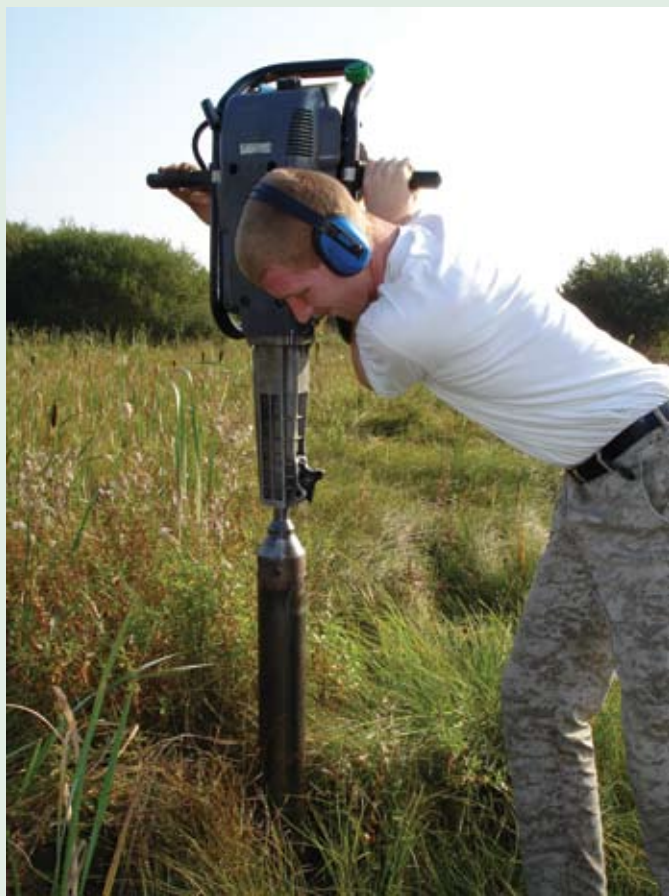
Fig 7: Soil sampling is an exhausting job, especially on heavy and stony soils. It takes a strong person to carry the 30-kg soil sampling equipment over long distances to the study sites, and it takes even more hands to carry back the soil samples. (Photo: M. Schrumpf)
