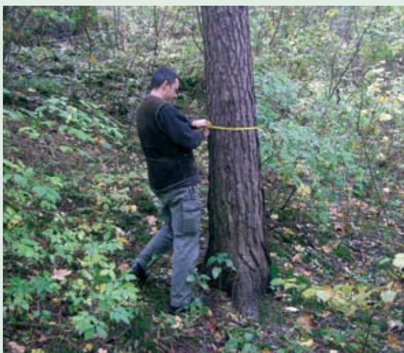
Fig. 16: Survey work in a forest in Germany. Mensuration of a) breast height diameter and b) stem position for future re-inventories. (Photo: D. Hessenmöller and M. Pöhlmann)
