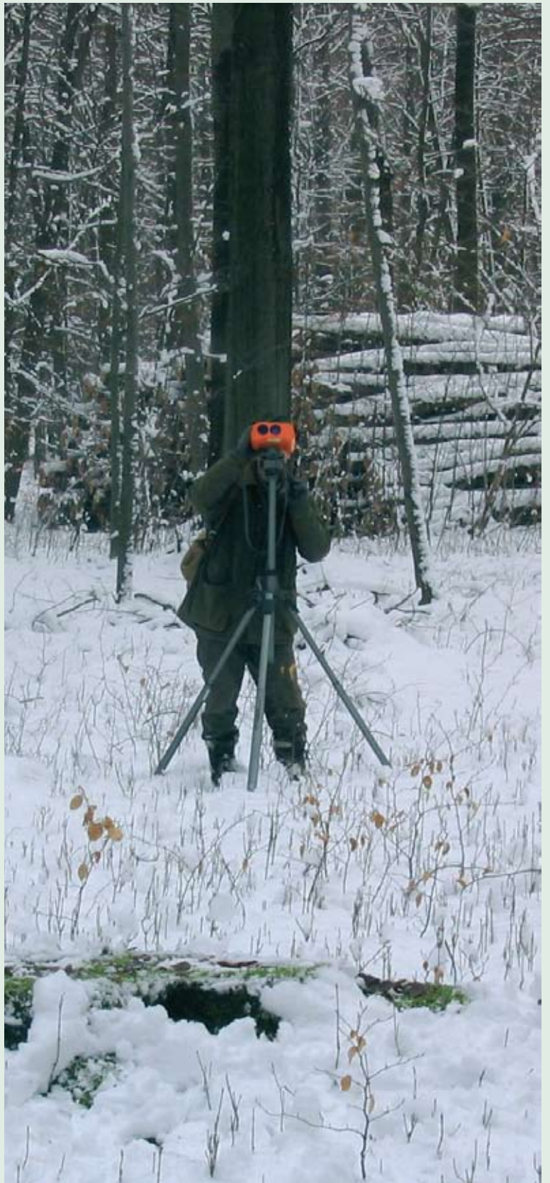
Fig. 16: Survey work in a forest in Germany. Mensuration of a) breast height diameter and b) stem position for future re-inventories. (Photo: D. Hessenmöller and M. Pöhlmann)
